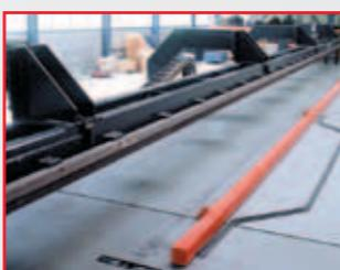
■ Automatic evacuation system to remove the finished products from the working plane.
