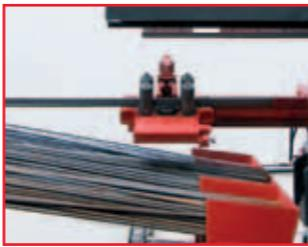
■ Semi-automatic pre-feeding unit for the alignment of the bars to be processed even during the work cycles.
