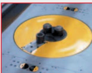
■ Single bending pin for the clockwise and anticlockwise bends.
