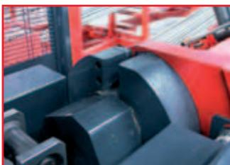
■ Shearing device consisting of universal cutting utensil useable for all the selected diameters.
