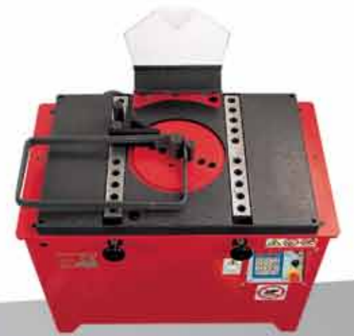
P 130 E To produce small and medium size stirrups and shapes.
