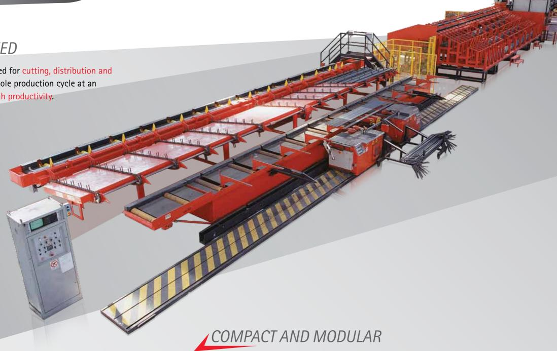
The **CUT LINE** uses a mobile holding rack, that aligns with the extraction feeding unit. The plant cuts the bars and unloads on both sides, being equipped with a large number of locations in the standard collecting racks as well as in the "two levels" automatic storage pockets. The **CUT LINE** operates with a substantial reduction of material transition phases, of the required plant footprint and also in the number of operators.
