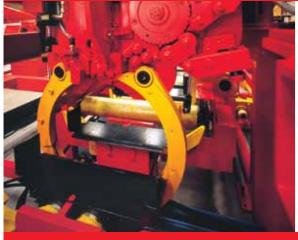
The automatic tying unit aligns and ties the cut to length bars.
