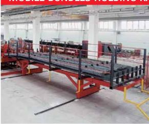
The mobile holding rack allows the bundles' storage within 7 or more compartments that depending on the diameter to be processed aligns to the (optional) automatic loading system reaching a continuous and automatic production cycle.
