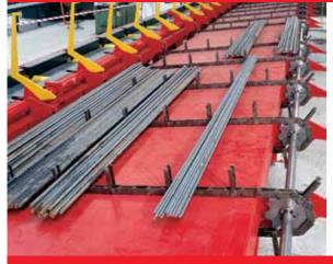
The chain feeder is a unit that collects, transports and deposits
