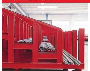
The storage rack is a unit that collects the bars cut to size automatically creating a large warehouse storage. CUT LINE, manages automatically every single job.
