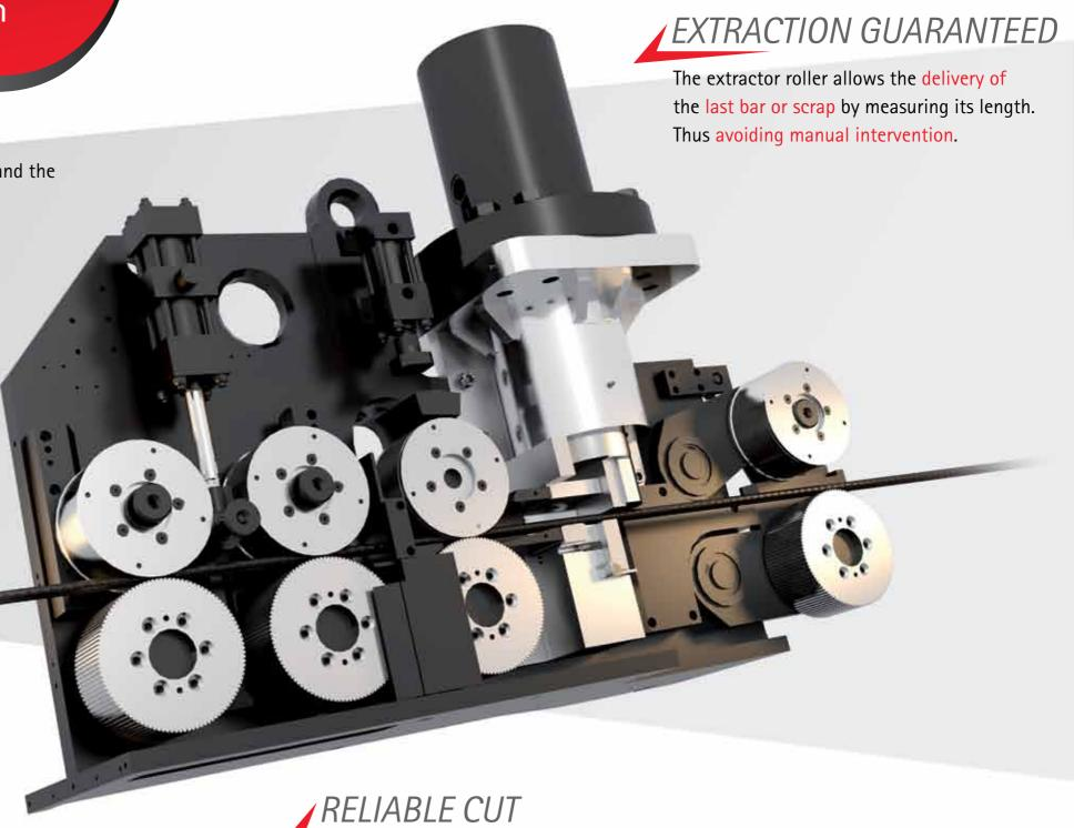
The hydraulic cutting system, normally used in the drop-down shear lines, has been chosen for its high reliability and cutting power.
