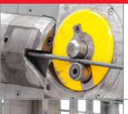
The cutting unit utilize universal mobile blade suitable for any wire diameter and provided with four cutting edges. Fixed blade guide dedicated by diameter.
