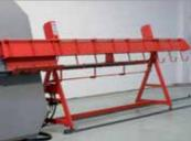
• Supporting and collecting unit for the production of straight bars and bars bent at one end.
