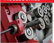
Motorized pre-feeding roller, for the insertion of the wires.
