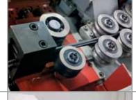
Motorized pre-feeding roller, for the insertion of the wires.
