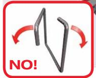
The twisting of the wire during the pulling phase creates open stirrups.
