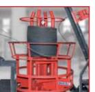
Spacer for the use of spooled or rewound coils. (OPTIONAL)
