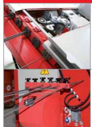
Multi-wire pre-feeding unit. Fully automatic, 6 positions for the wire changeover managed electronically by the control panel. (OPTIONAL)
