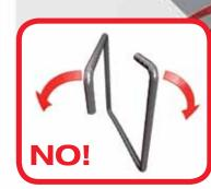
The twisting of the wire during the pulling phase creates open stirrups.
