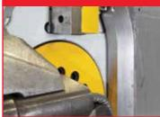
The three cutting units use universal knives, for all diameters processed with 4 cutting faces.
