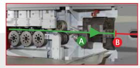
FORMAT LINE is equipped with a shear at "double effect" for the alignment of the initial part (head (A)) and end (tail (B)) of 2 bars.
