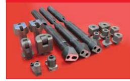
FORMAT LINE is equipped with a set of fast fitting bending pins. They are made in accordance with the international regulations, allowing the fast change during the diameter change phase, so the production can restart quickly.
