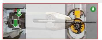
Generally the actual length of stock rebars is not known but always exceed the nominal theoretical of 12 or more meters (12,03/12,04m...). remove offcuts of any size.
