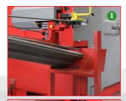
The use of the same feeding unit for the processing of the bar (1) and coil (2), allows to switch the production from one to another in a very short time. The straightening system "ARS" (Anti Rotation System) reconfigures itself in function of the type of material and diameter to be worked using the stored data.
