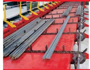
3 or 4-roller tracks). Their are moved transversally to the plant in order to create buffer of material and transfer the same to multiple areas equipped with bending tables (automatic or manual) and/or additional storage racks for cut to length material. (OPTIONAL)
