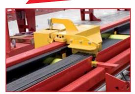
The bar length is obtained automatically through a mobile ledge device operating along the cutting track.
