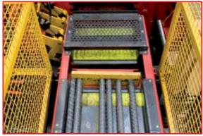
The modular bar-bundle storing racks, enable the storage of the bars on multiple levels (2 or 3 in standard configuration). The bars slide sideways at a lower level by mean of retractable arched arms. All bars are collected in a lateral pre-feeding channel which discharge them automatically onto the central feeding conveyor.
