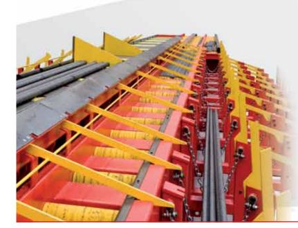
The roller conveyor positioned after the shear is equipped with two-speed motorized rubber rollers to transport the cut to size bars.
