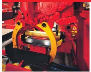
• The automatic tying unit aligns and ties the cut to length bars. Integrated within the LTM system eliminates the need for manual binding. (OPTIONAL)
