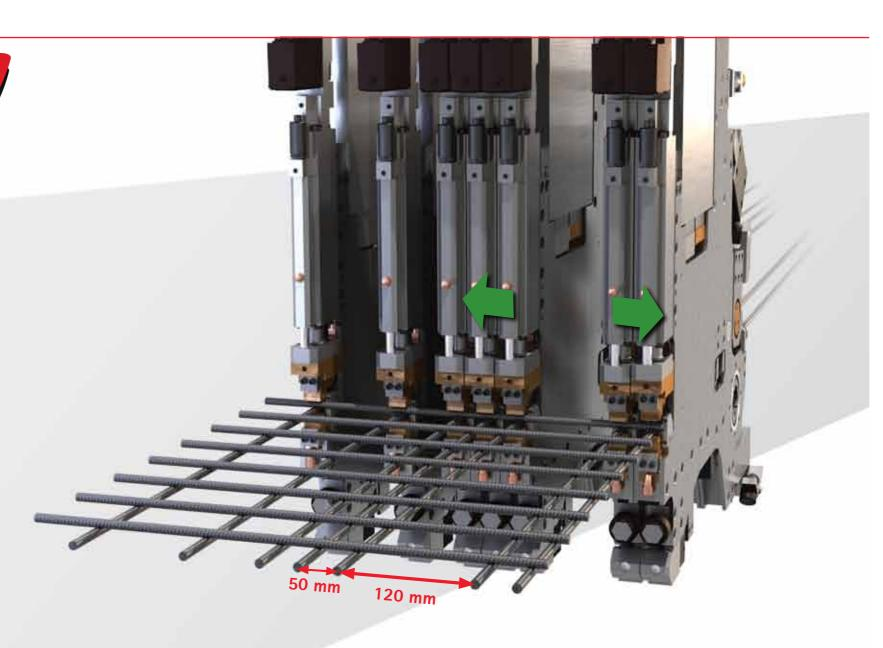
Semi-automatic pre-feeding module for longitudinal wires, equipped with storage table and led system for assistance in manual pre-loading operations.
