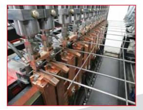
The MRSA M and MRSA S versions are welding machines equipped with an automatic loading system of the cross wires and "bridge cylinder" system with manual positioning of the welding units.
