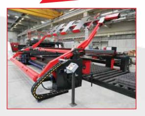
Automatic device for turning and stacking mesh panels.
