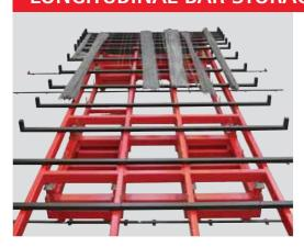
The bars storage table allows the stocking of longitudinal bar bundles for production purposes. (OPTIONAL)
