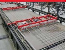
Produced panels can be fast-forwarded and ejected down to various final collecting stations according to customer's needs. Therefore the system can be equipped with one or more fastforward or ejection carriages or a blend of them to optimize working cycles. (OPTIONAL)
