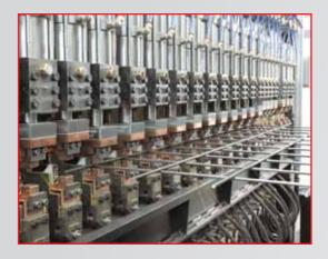
All MRSA welding plants adopt single welding press units with integrated transformers designed to be individually positioned at variable pitch distances.
