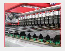
Automatic pre-feeding devices are able to count with accuracy and precision the position of each pre-cut bar.
