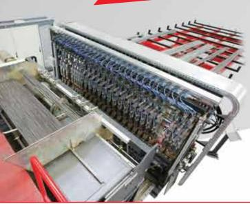
The MRSA Plants are designed to fit to a wide array of production requirements, processing fixed or variable pitch mesh (min pitch 25mm), with wire diameter ranging from 3-25mm. Stacking systems for panels and stocking systems for mesh panels can be specifically designed to suit the client and even adapted for upgrade of an existing plant at later stage.
