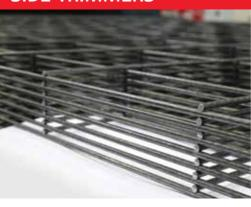
Cutting and trimming device for transversal protrusions (maximum diameter 8 mm) for the production of trimmed flat panels. (OPTIONAL)
