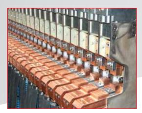
The MRSA SX Plant is based on a fixed welding head equipped with electronic programming system and manual positioning of the welding cylinders. It is designed to produce variable longitudinal pitches starting from 50 mm. The plant is equipped with a fully automated arrangement for the loading of both the long wires and the cross wires, thus allowing a fully automated production cycle.
