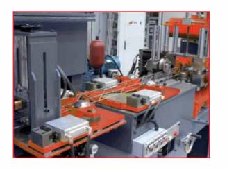
The feeding group is perfectly synchronised with the chain forming group so that the lattice girder will be produced in perfect symmetry.
