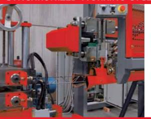
• The automatic transfer device of the lattice girder comes into operation after the cutting operation, thus enabling the production of next section.
