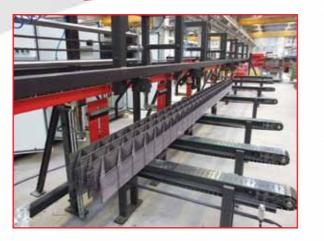
The finished lattice girders can be collected by means of an automatic stacking-machine that allows the material to be stacked according to the production and delivery plan.
