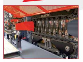
The vertical positioning of the chain forming groups is controlled by electric motors, so that it can be rapidly changed to match with any lattice girder height and wire size. It is an easy, precise operation having a very beneficial impact in reducing machine idle time. (MTM 400).
