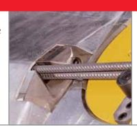
The cutting unit utilities universal knives for all diameters processed with 4 cutting faces.
