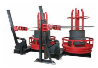
• **Decoilers** equipped with an automatic braking system monitored by the control panel according to the work cycle.
