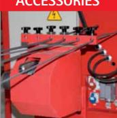
Winch equipped with clamping device for the wire end to be pulled.
