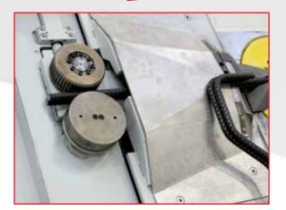
The extraction pulling unit reduces the scrap and eliminates the downtime needed for the extraction of the "tails", straightening and extracting automatically the final section of the coil.
