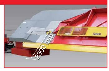
**PLANET 16 Plus** allows to get coplanar shapes and stirrups continuously closed, eliminating the dangerous manual operator intervention during the bending phase.
