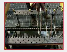
Identical cages can be produced without changes to the set-up. Reference pegs allow the operator to place the stirrups quickly in the required position.
