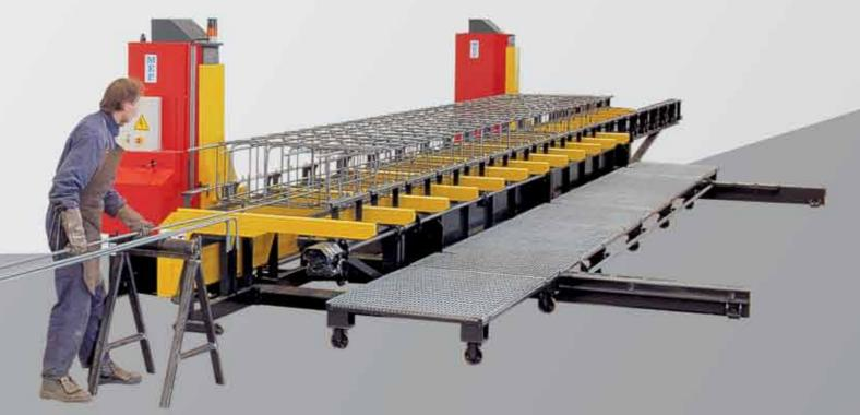
The lifting device allows the insertion and the support of the longitudinal bars or shapes at the height required, eliminating the need for a second operator. Intermediate heights can be obtained easily by means of a meter rule showing the heights.
