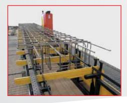
The positioning of the stirrups allows the operator to build cages in absolute safety, while preventing the excessive strain caused by lifting and supporting longitudinal bars.
