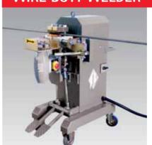
• Allows to weld the ends of two coils in order to reduce the handling time.
