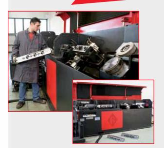
The straightening process is achived through a rotating group equipped with hyperbolic rollers having adjustable tilt and pitch. During the rotation phase, the wire is simultaneously dragged and straightened. This feature minimizes the longitudinal ribs deformation and does not affect the mechanical characteristics of the steel material. The use of dedicated rotors, depending on the various diameters, additionally improves the finished product quality.
