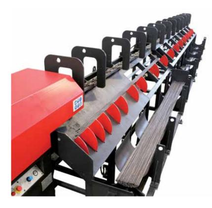
The guiding support available in several versions, allows the collection and separation of straightened bars according to their specific production needs.
