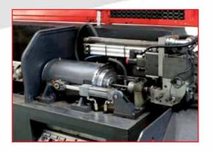
The flying shear cut to length the wire while is moving ensuring high speed performances and the respect of the measurement tolerances.
