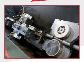
The insertion and straightening unit has an independent infeed that allows a constant control of the wire speed, originated by the hyperbolic rotor, based on the different diameters. An optimal quality of straightening is thus achieved.
