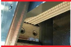
• The shearing unit uses universal blades for any diameter. Provided of 4 cutting faces.
