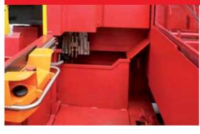
Mobile scrap bin mounted on rails to facilatate the removal.
