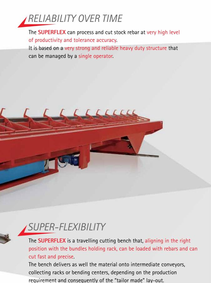
The modularity of a **SUPERFLEX** based plant, and in particular the
