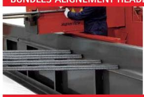
• Bundles alignment heading support for positioning and aligning the bars before insertion in the extraction/feeding group. (OPTIONAL)
