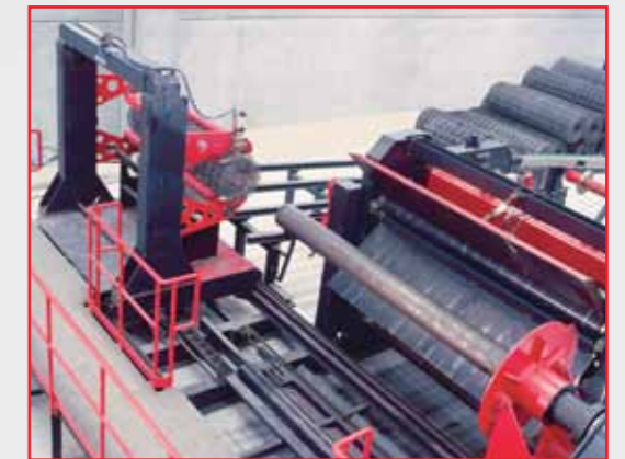
Withdrawing and off-loading automatic device.
