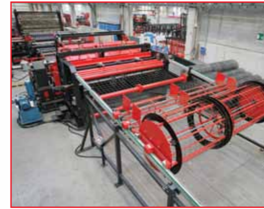
Buffer station of mesh in coil.
