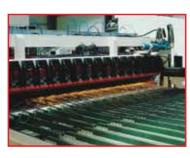
■ The universal welding unit (patented) is characterized by the adoption of a unique device which allows independent movement in both the vertical and horizontal planes of the individual welding pistons. This allows the realization of mesh elements with cross-wires positioned and welded either above or below the line-wires.
