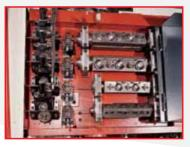
Multi-line straightening-and-cutting unit (cross-wires) with 4
