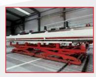
Evacuation cart and stacking of completed mesh elements.
