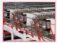
■ Chain device (patented) with automatic bar clamping devices for the independent placing (by number and position) of the line-wires.
