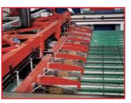
■ Mesh-expulsion device and transfer of mesh elements produced
